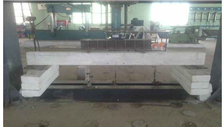
Fig -4: Testing of Beam specimens
