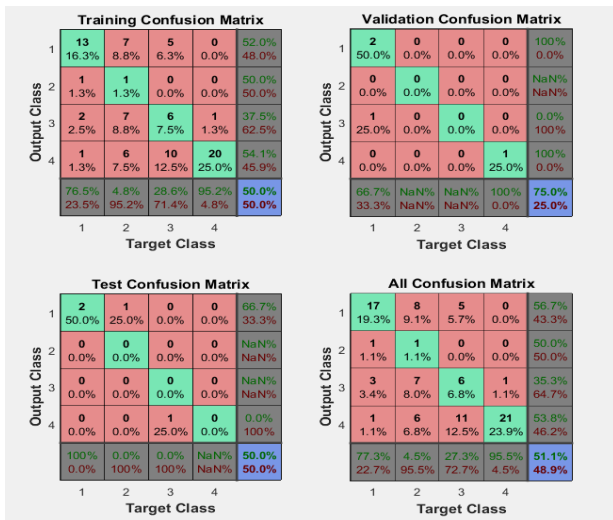
Fig-15: Confusion matrix for fault zone classification having efficiency 51.1%
