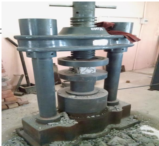
Figure - 4.0 Compressive test on concrete cube.
