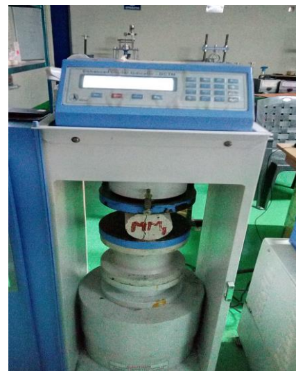
Figure - 5.0 Split Tensile strength test
