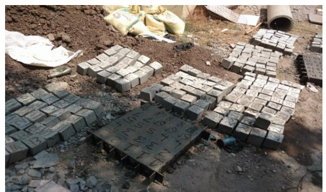
Figure - 3.0 Curing of Specimens
