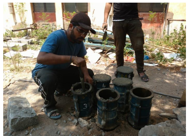
Figure - 2.0 Casting of Concrete Cylinders
