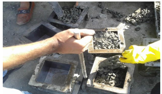
Figure - 1.0 Casting of Concrete Cubes
