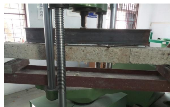
Fig 3: Initial Crack Formation e waste RCC beam
