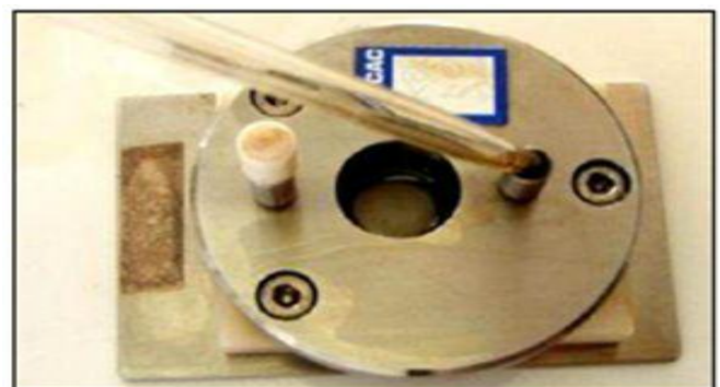
Figure 3: (a) Method M1: Thin film of asphalt on KBr pellets
