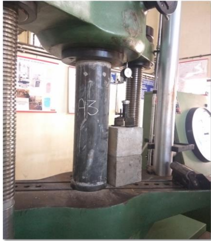
Fig -3: Experimental test setup of column specimens
