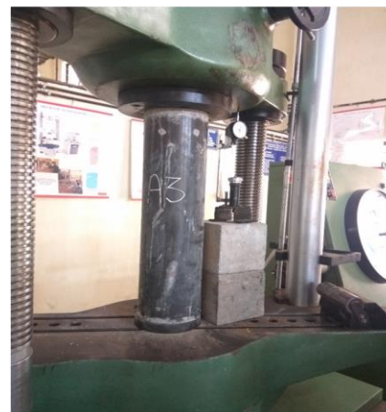
Fig -4: Experimental test setup of column specimens
