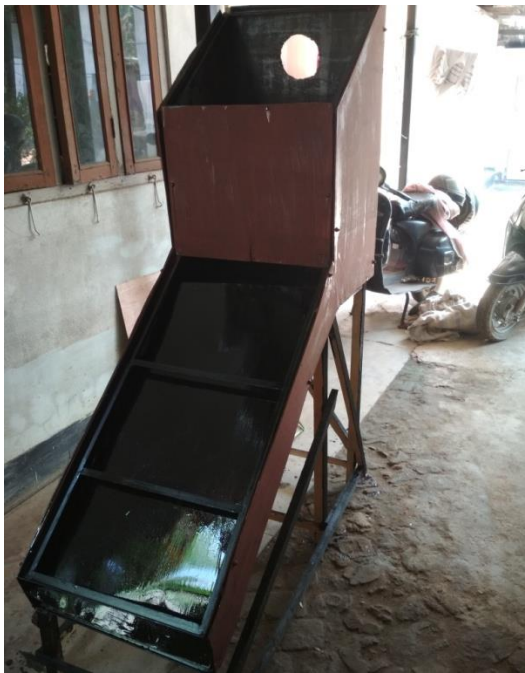
Figure 9: Painting black inside the dryer
