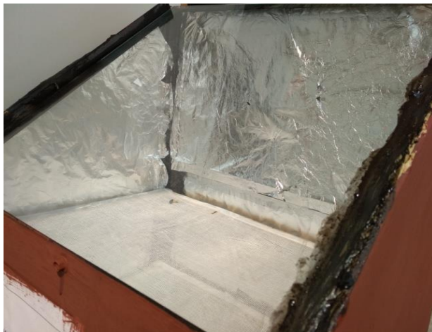
Figure 3: Top View of the solar dryer chamber
