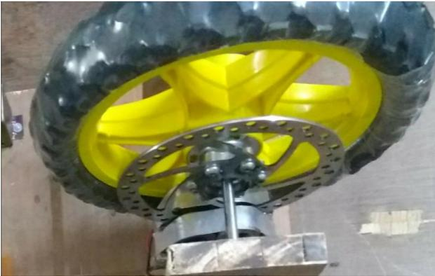
Fig-1: Wheel with electromagnetic brakes
