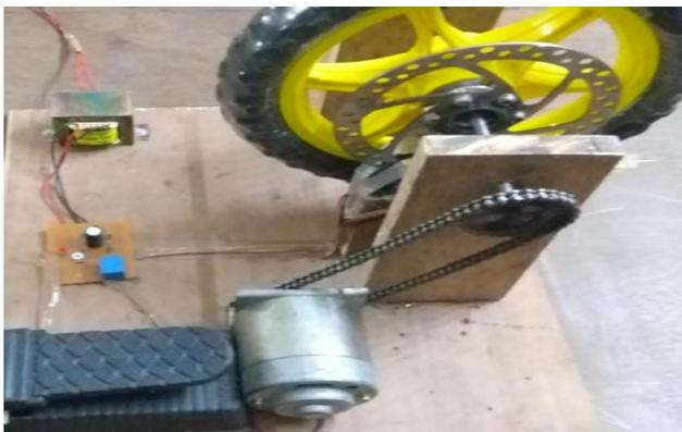
Fig-2: Electromagnetic braking arrangement
