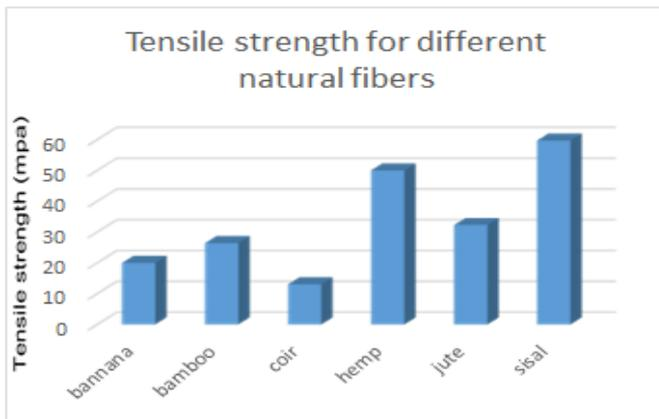
**Fig-1: Variation of tensile strength for different fibers**
