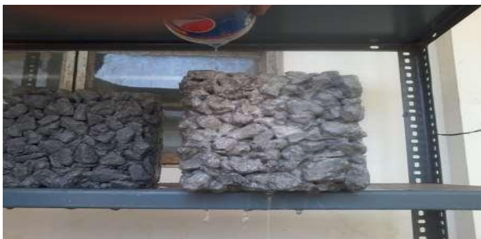
Figur1.3: water flowing through pervious concrete cube
