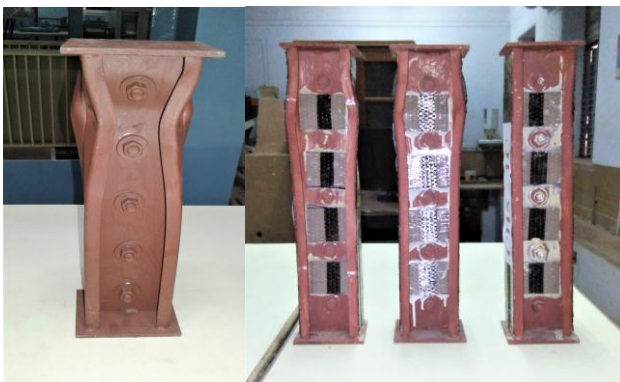
Figure 3 – Failure – Local Distortional buckling
