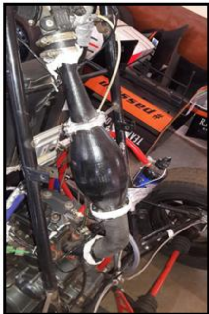
Fig 10. Final assembly of air intake
