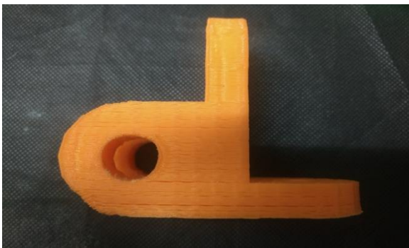
Fig. 4. layer splitting in specimen 3
