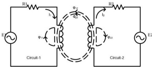
**Figure 1-** Inductive coupling with four Component Fluxes
