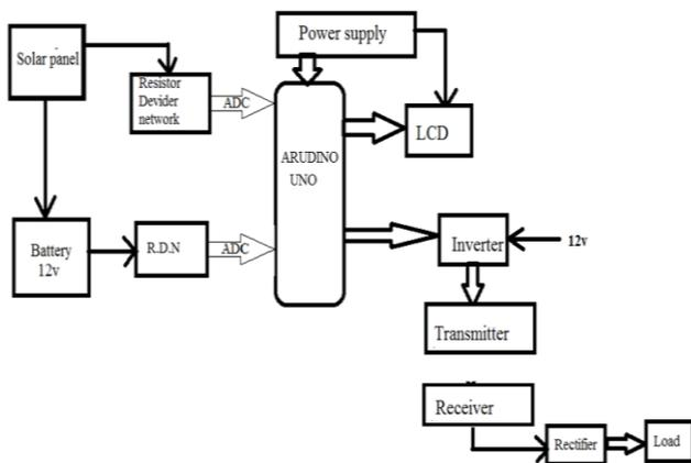
**Figure 2-** Block diagram for wireless power transmission via solar energy
