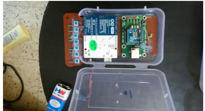
Fig-7: control circuit
