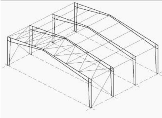
Fig-3: Horizontal Bracing System
