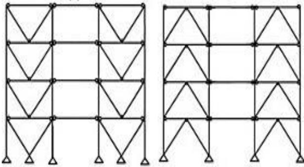
Fig-5: V Bracing
