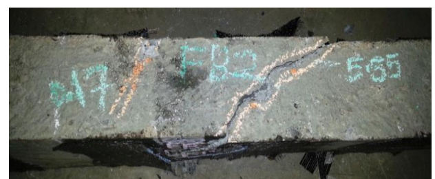
Fig 5.4 CFRP bonded RC beam before and after testing
