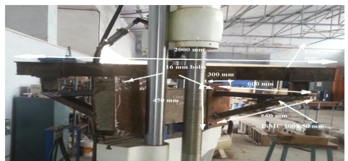
Fig 5.2 Torsion Testing Assembly
