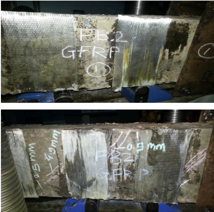
Fig 5.4 GFRP bonded RC beam before and after testing
