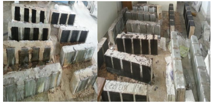
Fig 4.3 CFRP and GFRP bonded RC beam
