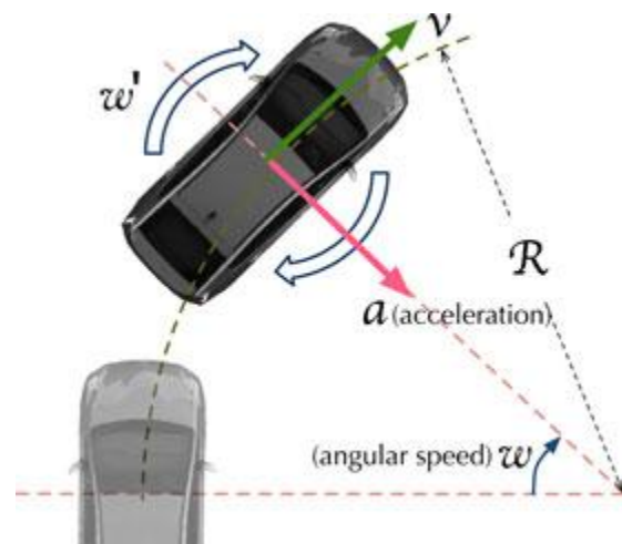
Fig -7: The circular movement detection when a car makes a turn via angular speed and acceleration.
