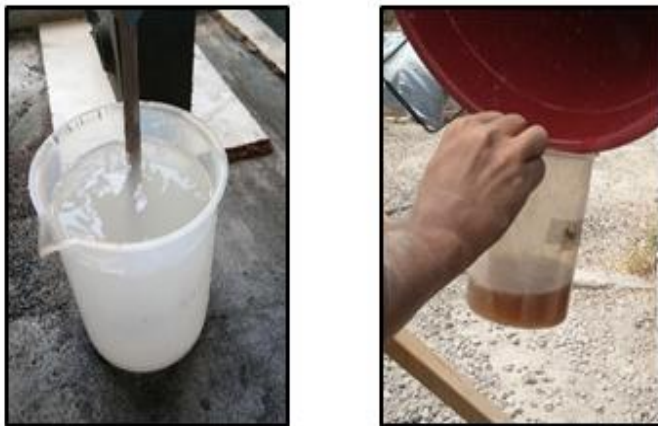
Fig. 4.1 Preparation of Alkaline Solution
