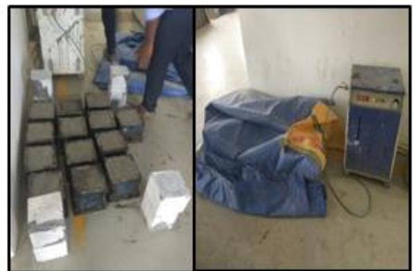
Fig. 4.4 curing of geopolymer concrete specimens
