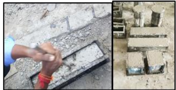
Fig. 4.3 Casting of geopolymer concrete specimens
