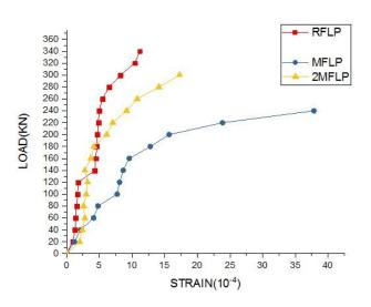
Figure 12: Strain variation across the mid-height FLC of panels at different load stages.
