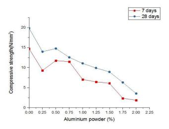
**Figure 6:** Compressive strength at different percentage of aluminium powder for 1:2 mix
