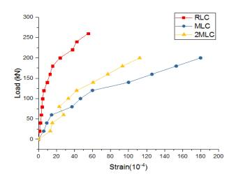
Figure 11: Strain variation across the mid-height of LC panels at different load stages.
