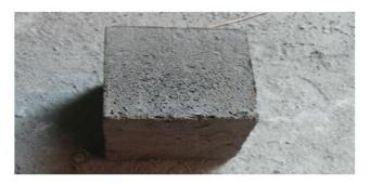
Figure 2: Lightweight concrete cubes
