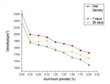
Figure 5: Densities at different percentage of aluminium powder for 1:2 mix
