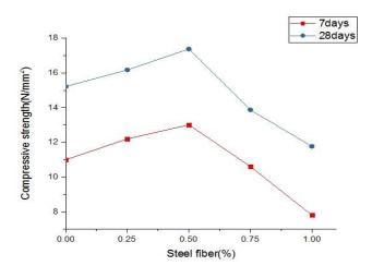
Figure 8: Compressive strength at different percentage of steel fibers
