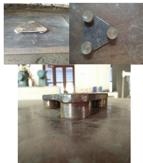
Fig 2 : Base plate used for the testing of Three stone column
