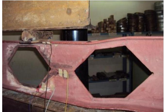
Fig -3: Flexure Buckling of Beam
