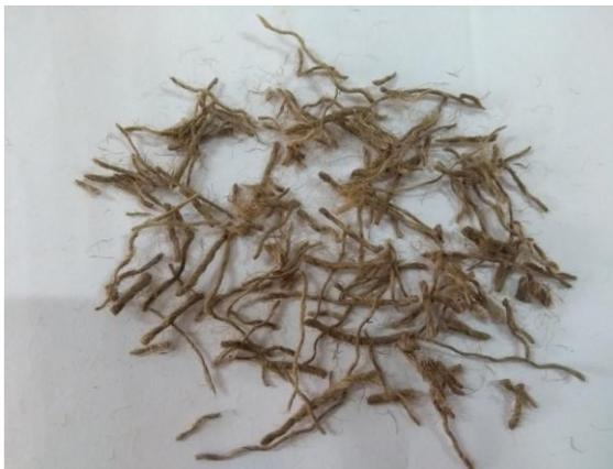
**Fig-16:** Jute fibres cut in lengths of 10mm
