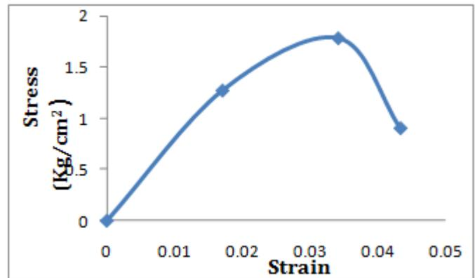
Chart -2: Stress – strain graph from UCS test without reinforcement
