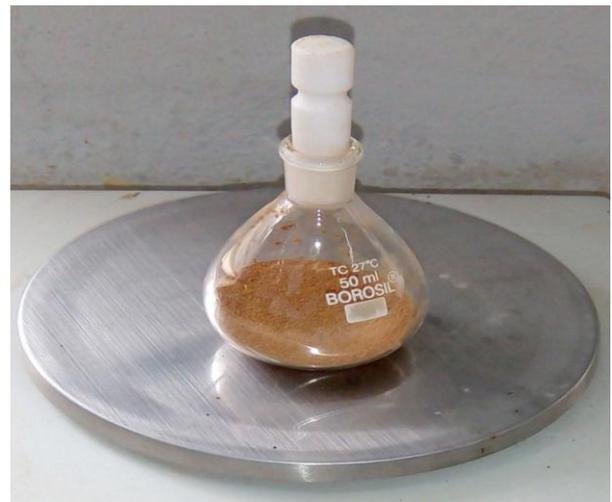
**Fig-8:** Specific gravity test
