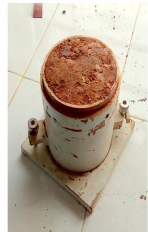
**Fig-10:** Proctor mould with compacted soil
