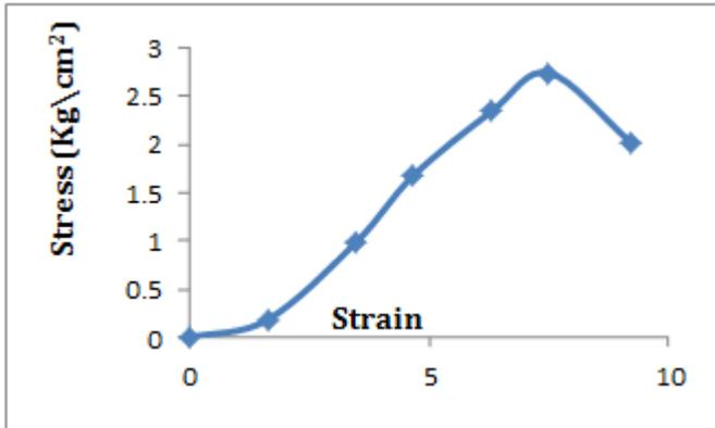
Chart -3: Stress – strain graph from UCS test using jute fibres
