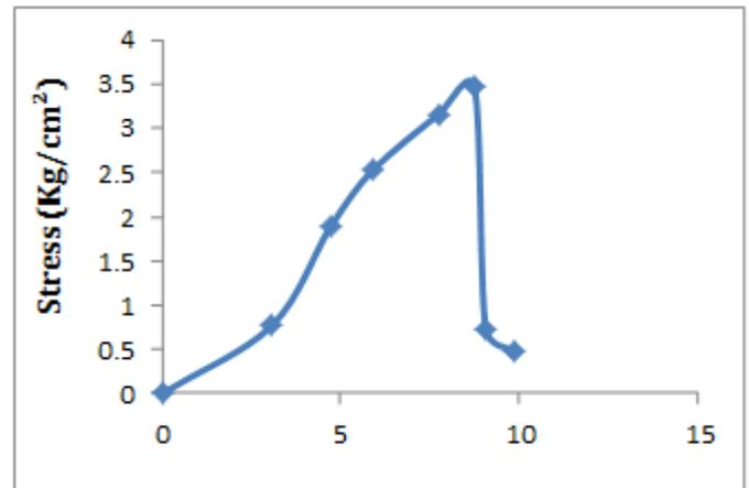
Chart -5: Stress – strain graph for jute layers coated with bitumen placed simultaneously in the sample
