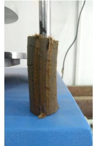
**Fig-14:** Sample at failure for 2% jute
