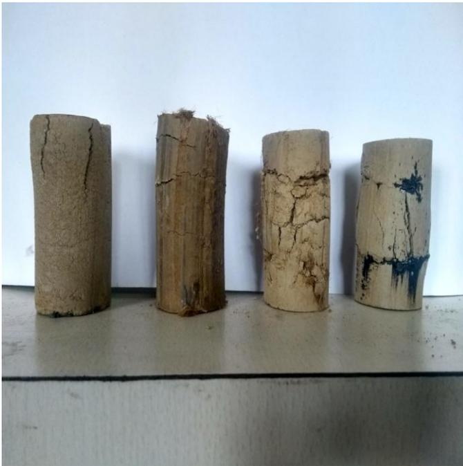
**Fig-24:** Failed samples (from left) of unreinforced soil, with 2% jute fibres thoroughly mixed, with three layers of jute placed simultaneously, with three layers of jute coated with bitumen placed simultaneously
