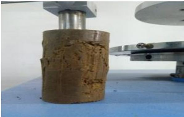
Fig-19: Sample after failure
