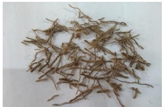
**Fig-3:** Jute fibres
