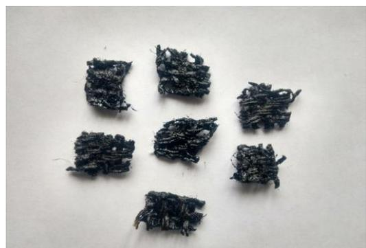
**Fig-4:** Jute layers coated with bitumen.
