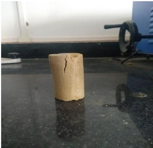
Fig-15: Failed soil specimen
