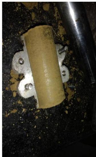
Fig-13: Soil specimen for Ucs test
