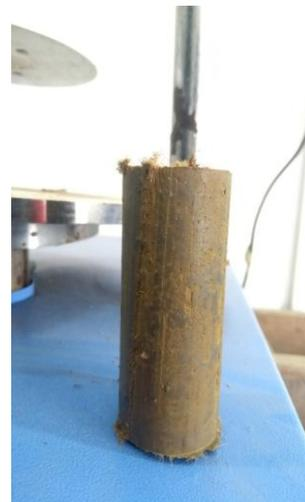
**Fig-13:** Sample before failure for 2% jute
