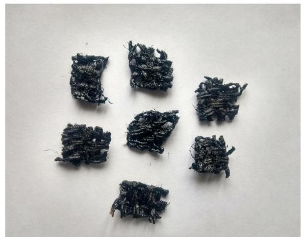
Fig-20: Jute layers coated with bitumen
