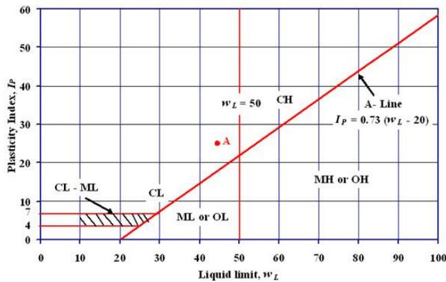
**Fig-11:** Plasticity chart as per Indian Standard Soil Classification system
