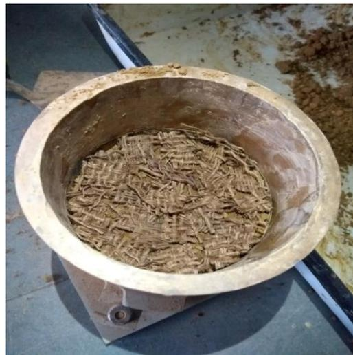
Fig-16: Preparation of sample with jute layers
