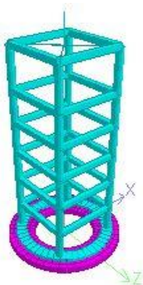
Figure - 2.2 Model geometry of staging part and plate model with annular raft in staad pro V8i.
