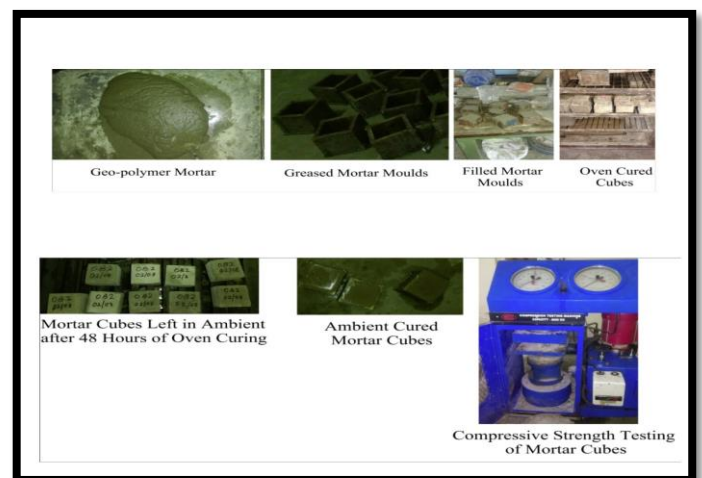
Fig -3: Preparation, curing and evaluation of compressive strength cement free fly ash based geopolymer mortar
