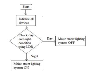
Fig -2: Flowchart for checking day and night condition using LDR
