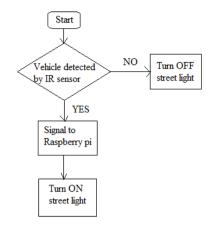
Fig -3: Flowchart for vehicle detection
