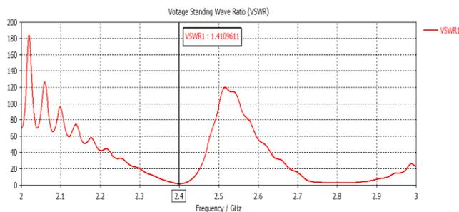
Fig -6: VSWR of alumina substrate
