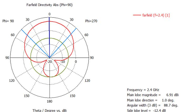
Fig -9: Directivity of paper substrate
