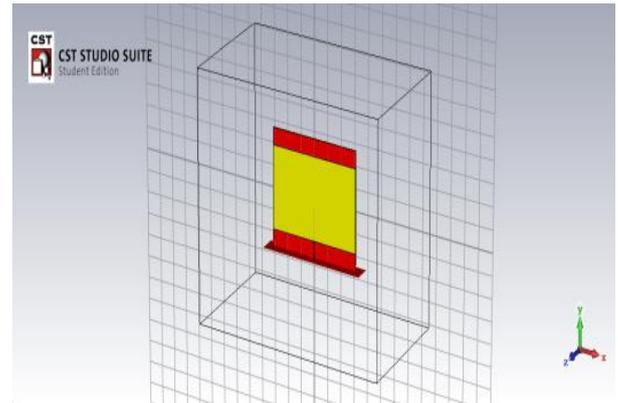
**Fig -3:** Geometry of rectangular microstrip patch antenna using paper substrate.
