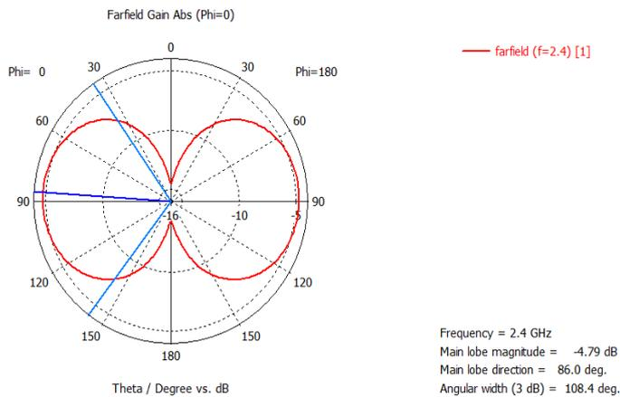
Fig -10: Gain of alumina substrate
