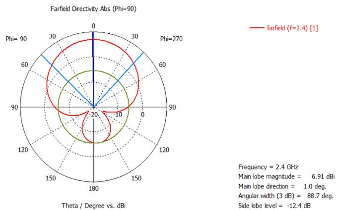
Fig -8: Directivity of alumina substrate
