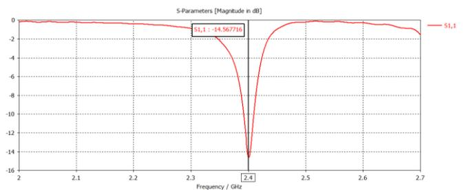
**Fig -4:** S11 Parameter of alumina substrate
