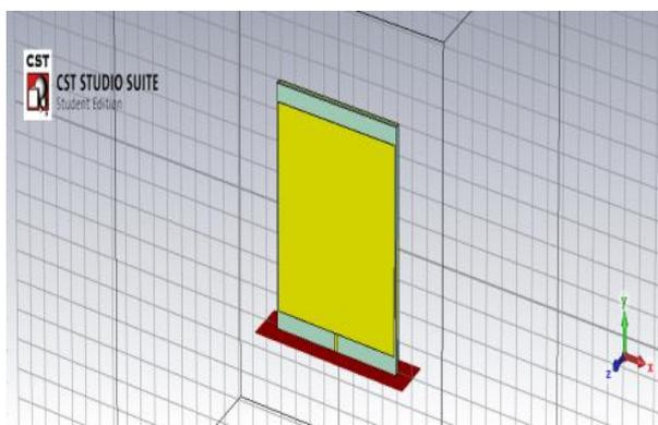
**Fig -2:** Geometry of rectangular microstrip patch antenna using alumina substrate.
