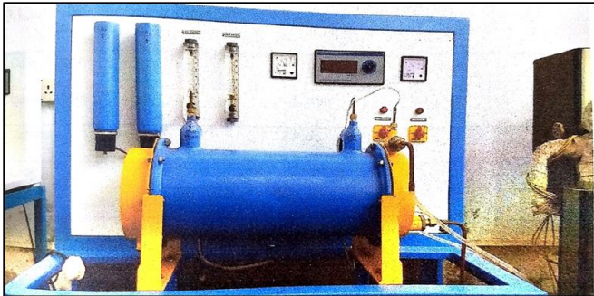
Fig -3.1: Experimental setup of shell and tube heat exchanger
