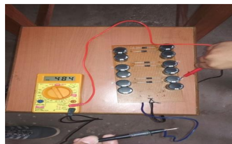
Fig 4.2 First stage output (484v)
