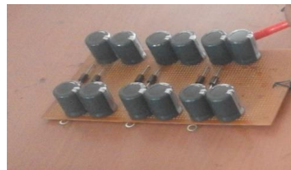
Fig.4 Hardware setup Cockcroft-Walton voltage multiplier circuit
