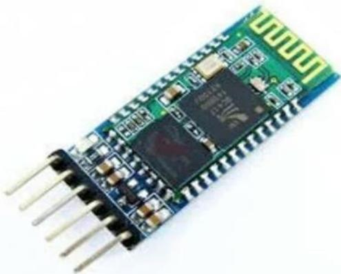
Fig-3: Bluetooth Transceiver Module
