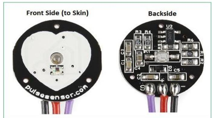
Fig -1: Pulse Sensor
