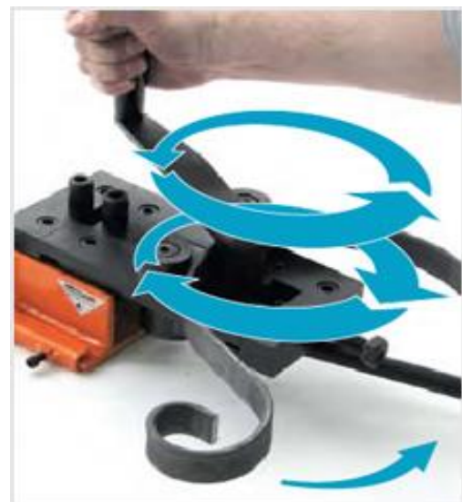
Fig - 5: Rolling Operation
