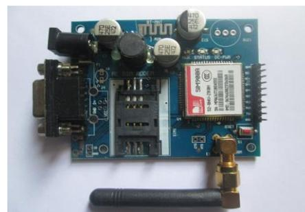
**Fig- 6: GSM Module**
