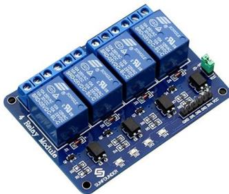
Fig.3 Channel 5v Relay Modules
