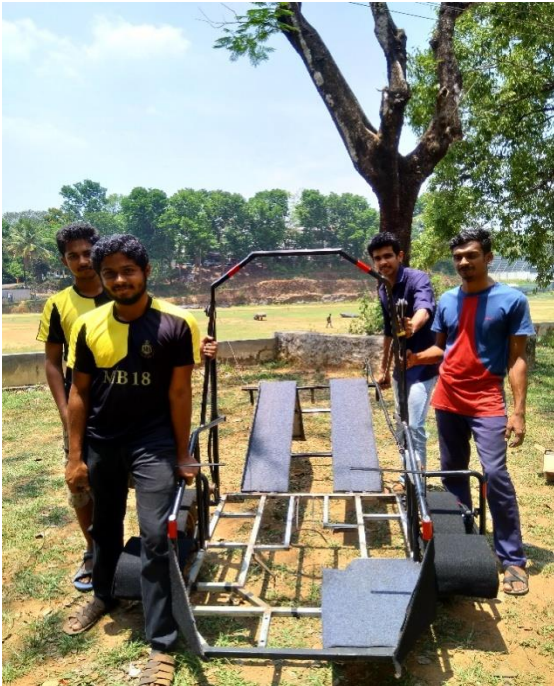
Fig21: Wheel chair Accessing mechanism for scooter
