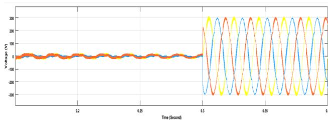
Figure 3.6 Load side voltages with respect to time of Shunt Hybrid Filter
