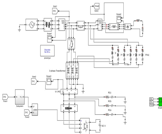
Figure 4.5 MATLAB Model of Series Hybrid Filter
