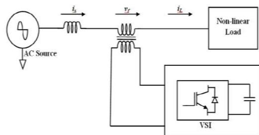
Figure 2.5 Circuit Diagram of Series active power filter
