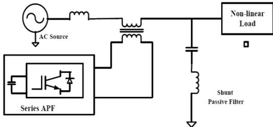
Figure 2.10 Series APF with Shunt Connected Passive Filter
