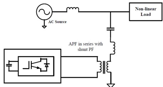
Figure 2.9 APF in series with Shunt Connected Passive Filter
