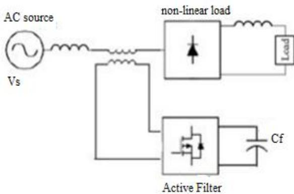
Figure 4.3 Basic Compensation Principle of Series Active Filter
