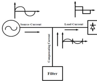
Figure 1.1 Basic Operation of Filter
