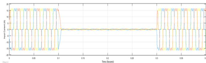
Figure 3.5 Input Current with respect to time of Shunt Hybrid Filter
