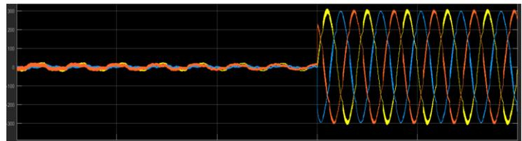
Figure 4.8 load side Voltage with respect to time of Series Hybrid Filter
