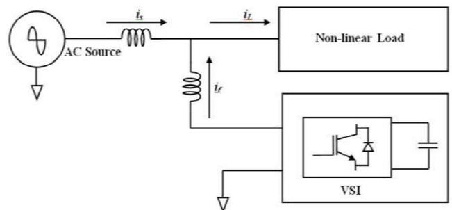
Figure 2.4 Circuit Diagram of Shunt active power filter
