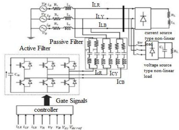
Figure 3.1 System Configuration
