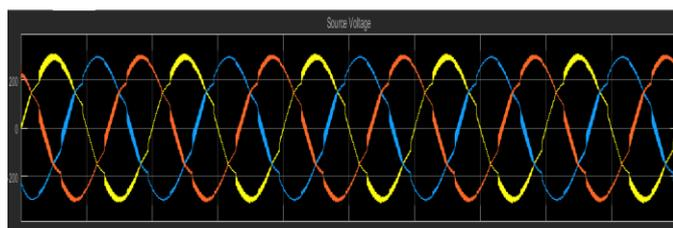
Figure 4.6 Input Voltage with respect to time of Series Hybrid Filter
