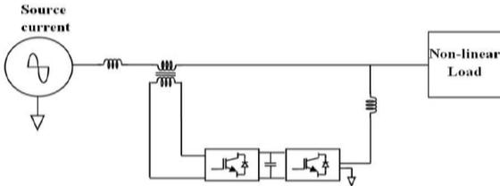
Figure 2.6 Circuit Diagram with UPQC
