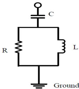
Figure 2.3 High Pass Filter
