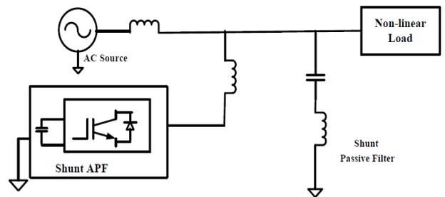
Figure 2.8 Shunt APF and Shunt Passive Filter Combination
