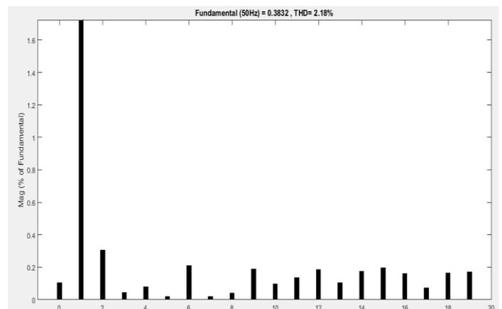
Figure 4.10 FFT analysis of Series Hybrid Filter
