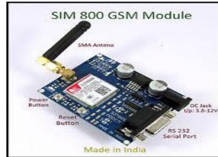
Fig - 3: GSM Module
