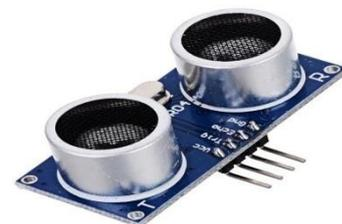
Fig - 4: Ultrasonic sensors
