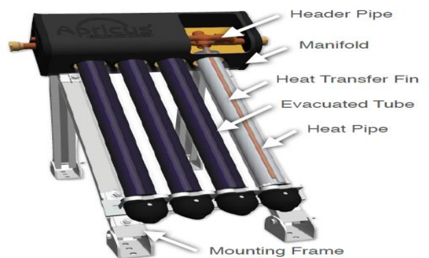
Figure 3. Evacuated Tube Solar Collector
