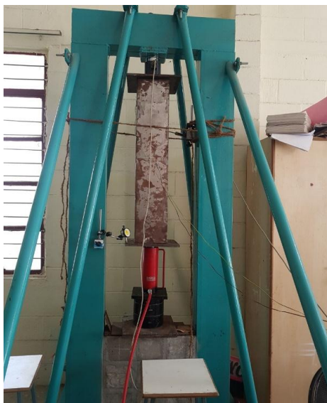
FIG 4: EXPERIMENTAL SET-UP FOR FACE TO FACE SPECIMEN
