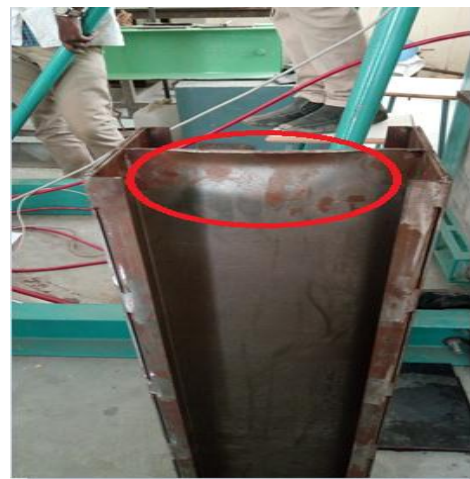
FIG10: FAILURE OCCUR AT THE BOTTOM OF FACE TO FACE SPECIMEN
