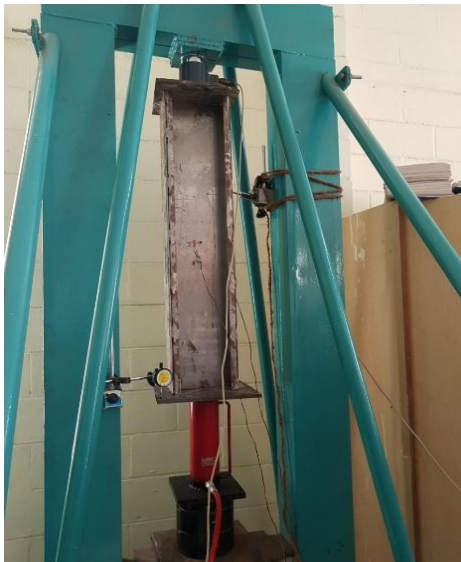
FIG 4: EXPERIMENTAL SET-UP FOR FACE TO FACE SPECIMEN
