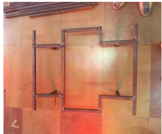
Figure 4:- Completely welded chasis.
