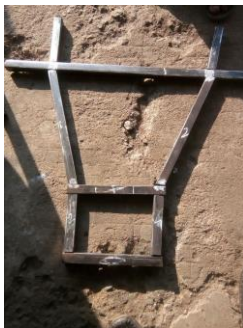
Fig- 4.1.1: Chassis (Frame) before welding
