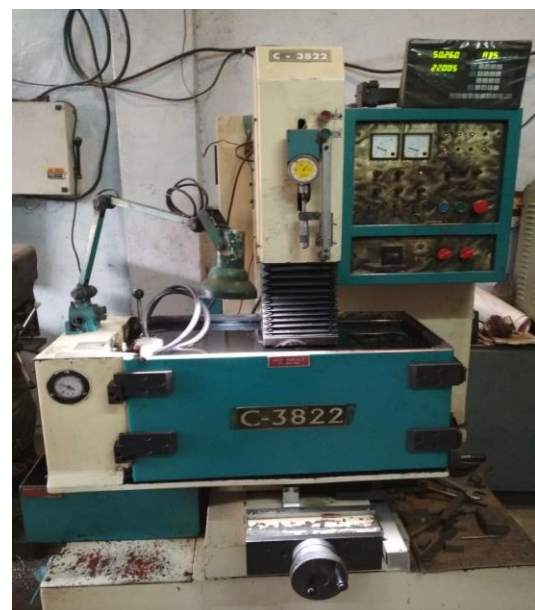
Fig -4: EDM used for drilling process
