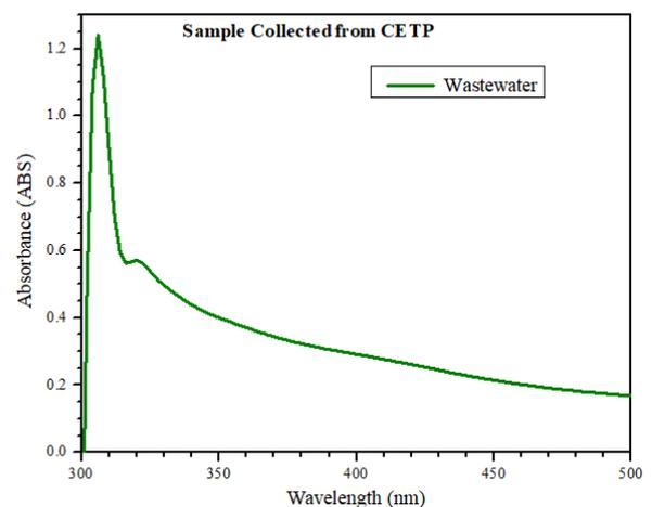
**Fig 2:** Wastewater Characterization Using Uv-Spec.
