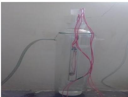
**Fig 1 :** UV Reactor setup
