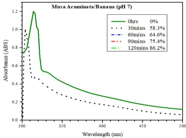
**Fig 7:** Absorbance Of Wastewater At Ph 7 For 30 Mins
