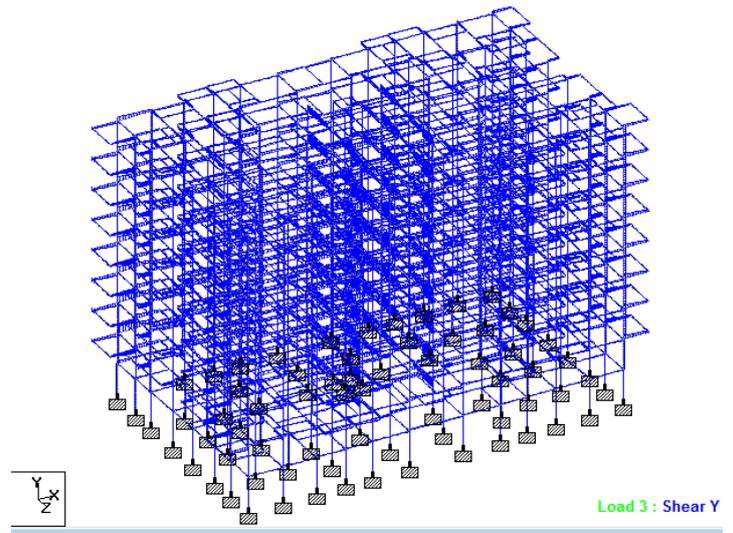
Fig. - 4: Shear in Y-Direction
