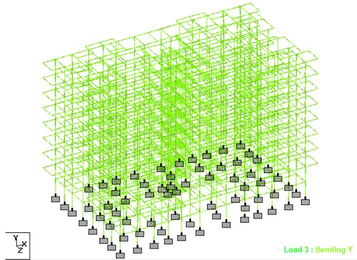
Fig. - 5: Bending Moment Y-Direction
