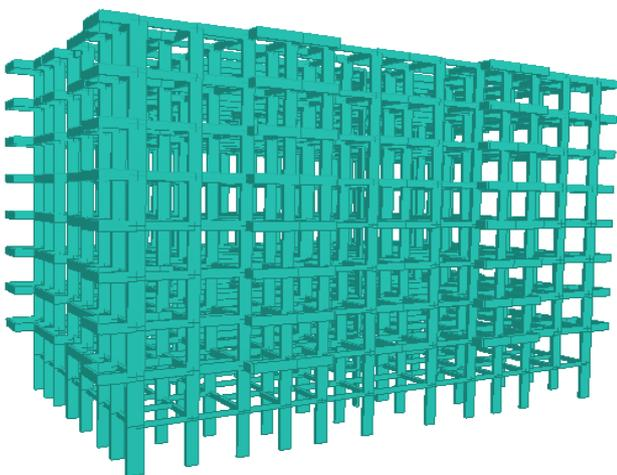
Fig. - 3: 3D model of building generated in Staad.pro.v8i
