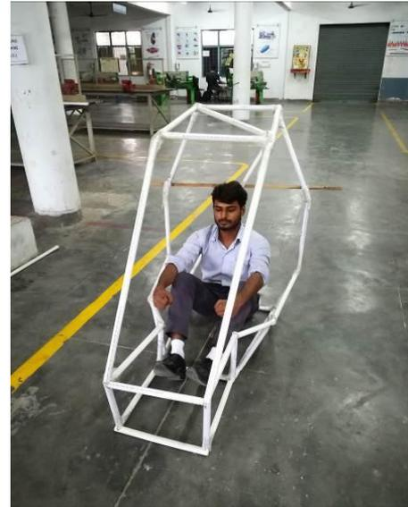
Figure 2: Checking the ergonomics of the frame
