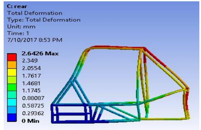
Figure 6: Maximum deformation in Rear impact
