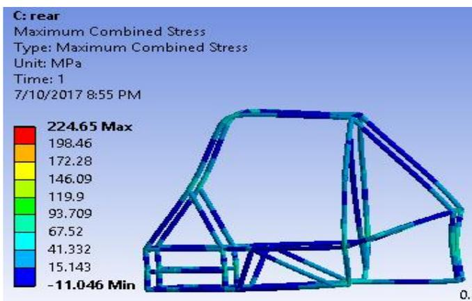
Figure 5: Maximum Stress in Rear Impact
