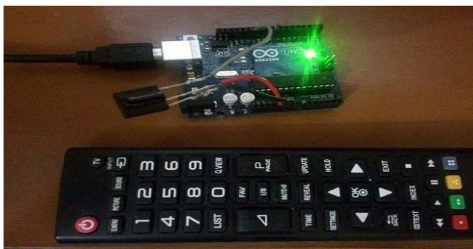
Fig-2 Arduino IR receiver interface
