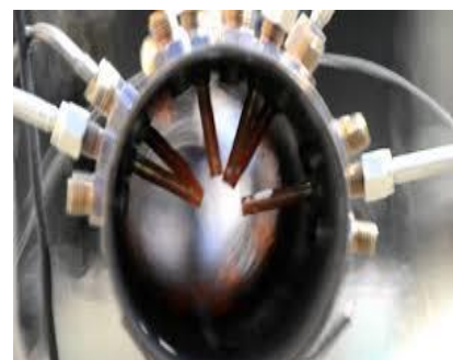
Fig 2:-Thermocouple Installed In Aero-engine Component
