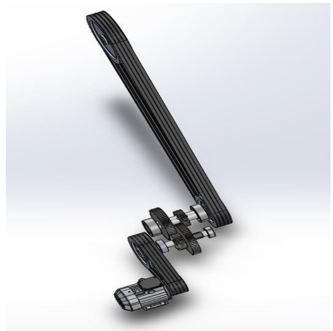
Fig.2.3.1 3D model of gearbox
