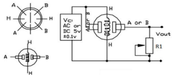
Fig2. Sensor is connected in series with a variable resistor to form a voltage divider circuit
