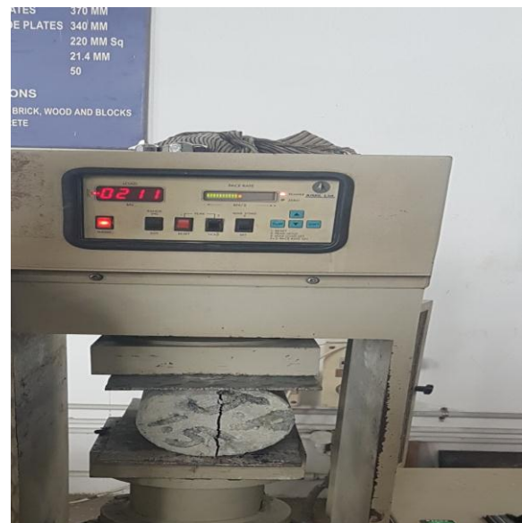
Fig. 1.2 split tensile strength test
