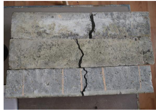
Fig 1.6 Specimen After Testing
